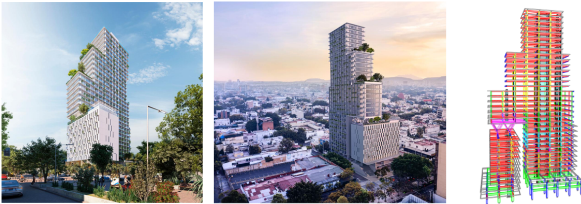
Figure 1. Render view of the building locating in Mexico(right) 3D ETABS model of the building (left)
